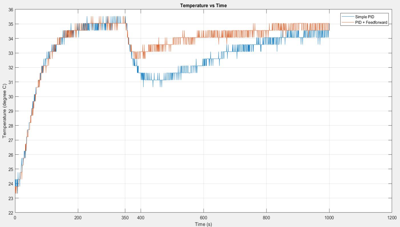
**Key Observations:** (1) *Blue line (Simple PID)*: Sharp drop to  $\sim 31^\circ\text{C}$ , slow recovery. (2) *Orange line (PID + FF)*: Minimal drop to  $\sim 33^\circ\text{C}$ , rapid recovery. Feedforward preemptively adds heater power instantly when fan turns ON, preventing most temperature deviation. PID alone only reacts after observing error.
