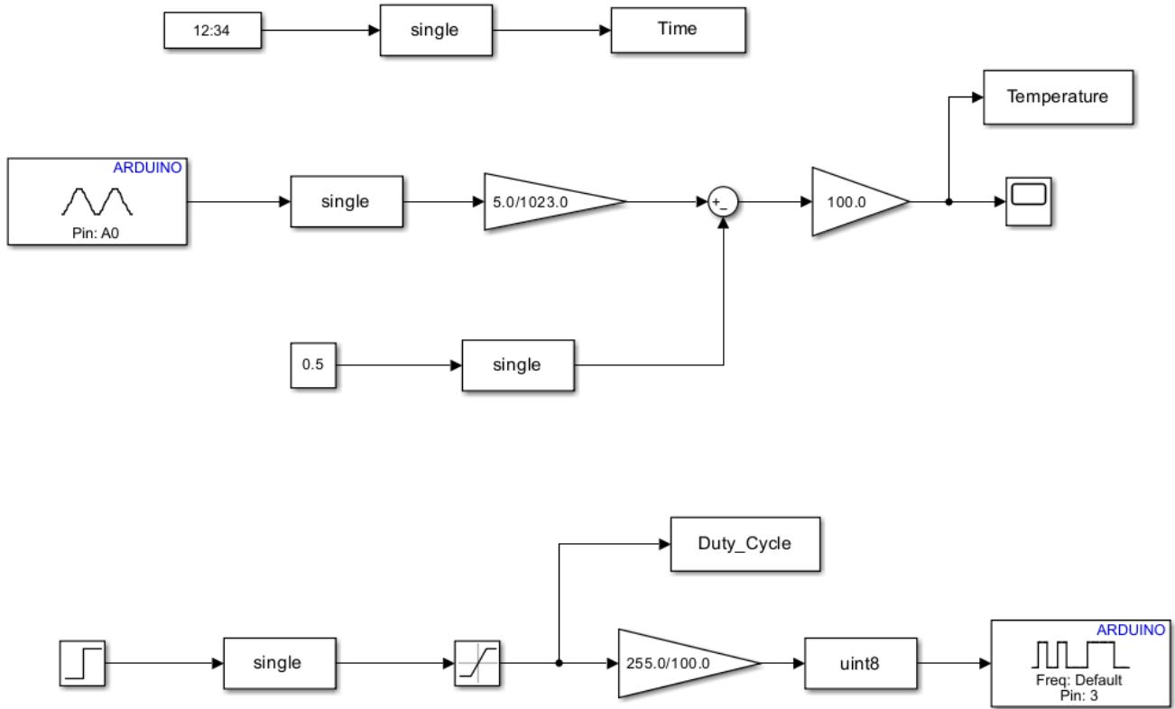
B The following Simulink model was used to first do simple PID control (Feedforward was commented out) and then with feedforward control. During Feedforward control, press button was used to turn the feedforward gain ON at same time when fan was manually turned ON at 350 sec.
